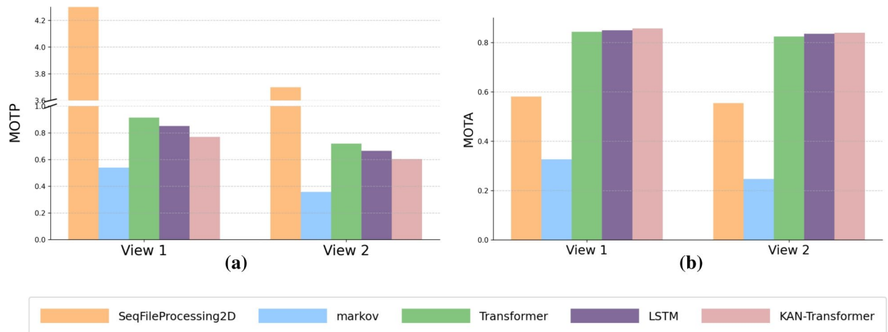
Fig. 4. Tracking Performance comparison between KAN-Transformer and other methods in two orthogonal views of the dataset. The dataset comprises 700 frames with 400–500 flies. (a) MOTP: lower values indicate better performance; (b) MOTA: higher values indicate better performance.
