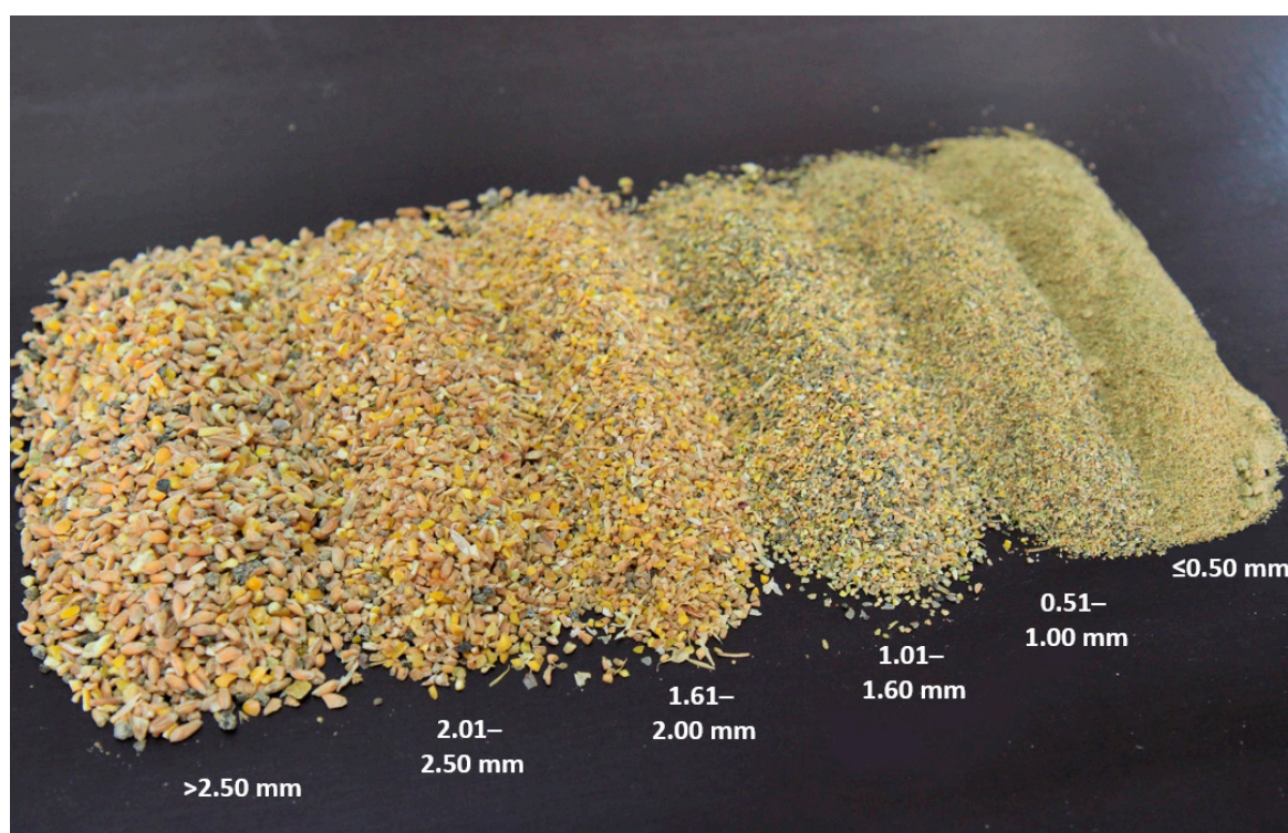
Figure 1. Feed particle fractions after a sieve analysis of a laying hen complete diet.
