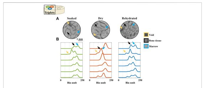
**FIGURE 4** | Histograms of the neutron tomography images of the trabecular bovine bone plugs. **(A)** Transverse slices of representative specimen from each hydration group. **(B)** Specimen-specific histograms. Each line corresponds to one specimen (*n* = 6 per hydration group). Each row corresponds to one triplet, i.e., plugs extracted next to each other from the same anatomical location. Arrows indicate peaks corresponding to void (yellow), bone tissue (black), and marrow (blue).
