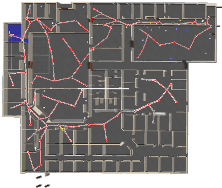
Figure 1. Result of autonomous exploration and mapping of the Willow Garage office environment using the proposed method. The resulting graph for the mapped area is overlapped over the Gazebo environment.
