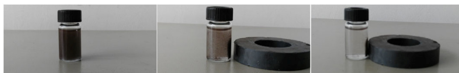
Figure 2. Separation process of adsorbents under an external magnetic field from left to right.
