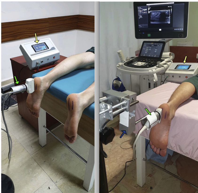
Fig. 3. A. The position of the ultrasound probe connected to the dynamometer targeting the heel of the patient in the prone position. B. Ultrasonographic measurement of heel fat pad thickness under constant pressure. (yellow arrow, dynamometer display; green arrow, ultrasound probe; blue arrow, dynamometer sensor.)
