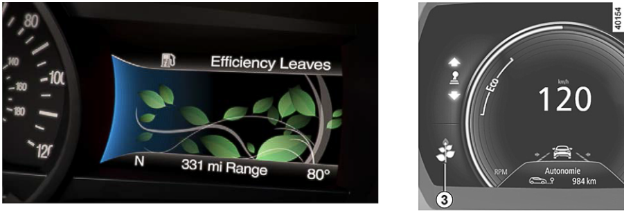
Abb. 2 Ford Dashboard mit EcoGuide (Quelle: Ford EcoGuide, https://owner.ford.com/support/how-tos/vehicle-features/dashboard-instrument-cluster/smartgauge-with-ecoguide.html ) und Renault Driving Style Indicator (Quelle: Renault driving advice, eco-driving: https://gb.e-guide.renault.com/eng/Kadjar/DRIVING-ADVICE-ECO-DRIVING )
