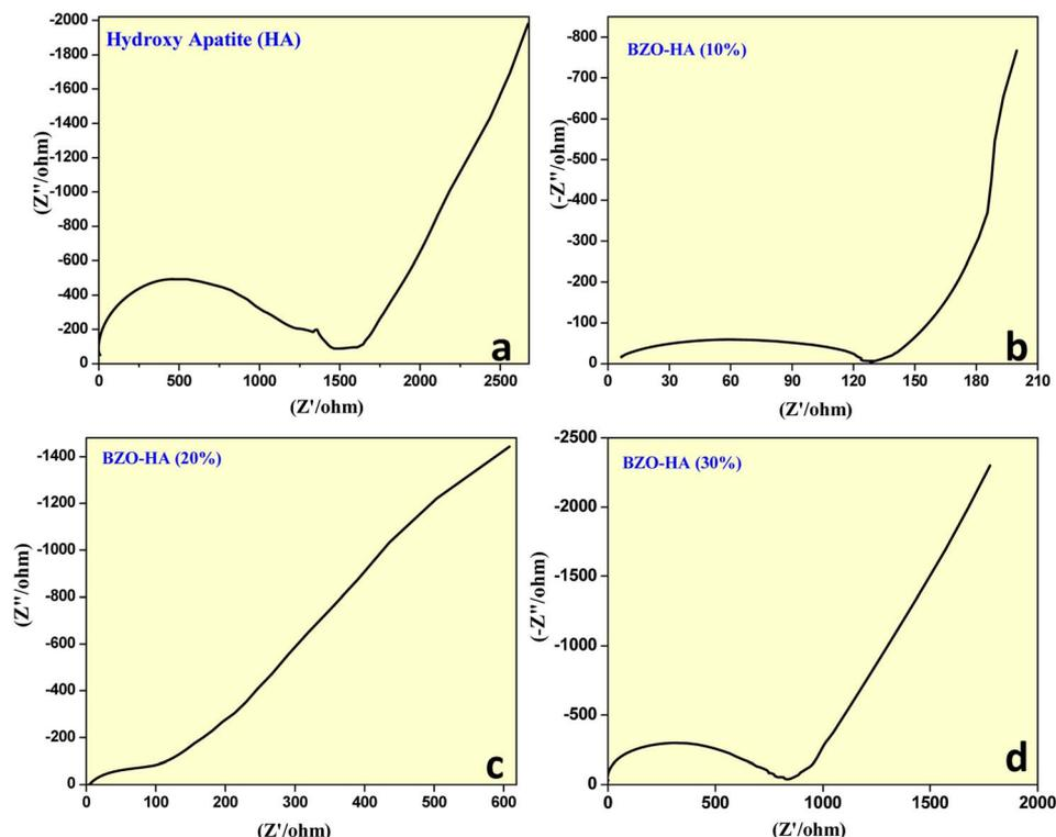
Fig. 8 Nyquist plots for HA and BZO-HA (10%, 20% and 30%) nanocomposites at various scan rates.
