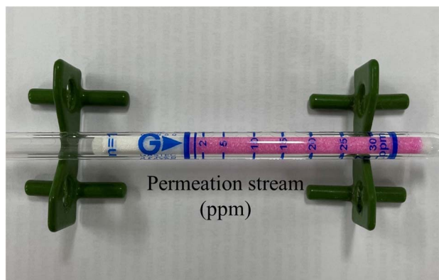
Fig. 8 Ammonia concentration in the permeation stream measured by a gas detector during the ammonia decomposition test using a membrane reactor at 748 K with a retentate stream gauge pressure of 150 kPa, a permeation stream vacuum of -10 kPa, and an ammonia feed flow rate of 12 000 mL min -1 .
