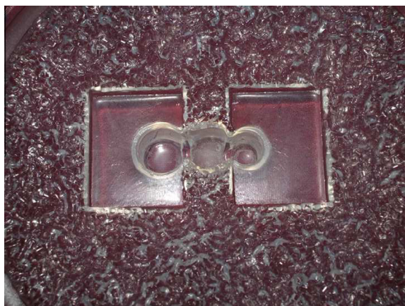
Figure 2 Template used to make the wax pattern of the test specimen.
