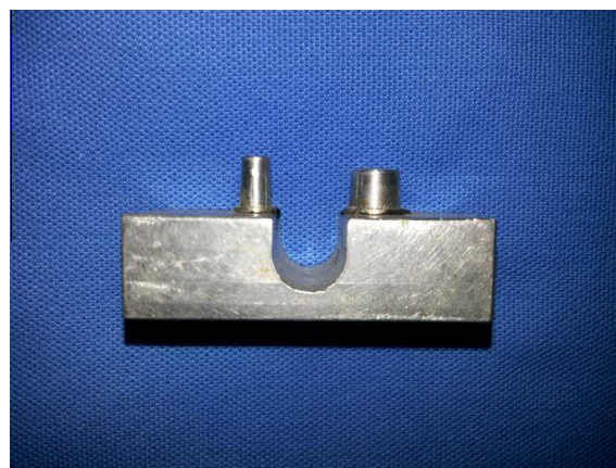
Figure 1 CAD CAM die simulating fixed partial dentures.
