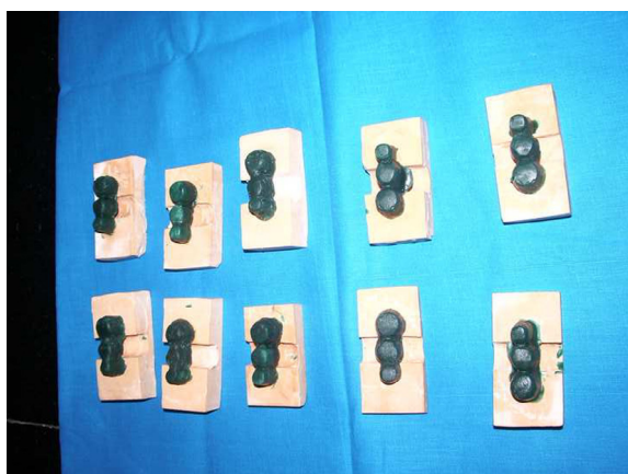
Figure 3 Wax pattern of the sample on the die stone cast.
