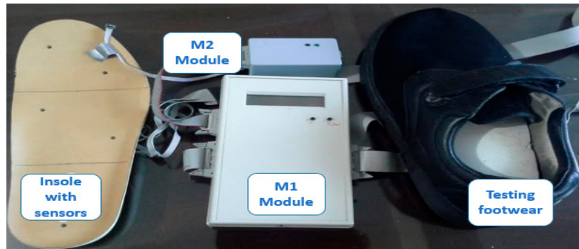
Figure 6. Prototype of the portable system for monitoring the microclimate in the interface of foot, footwear, and insole with sensors.
