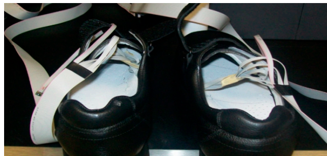
Figure 7. Array of ten sensors placed on flexible cables in the footwear.
