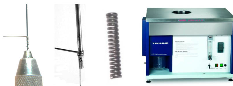
Figure 2. The production process of the NiTi spring. In this process, a NiTi wire is first wrapped around the NiTi wire, and then the shape setting procedure is performed to create the spring.
