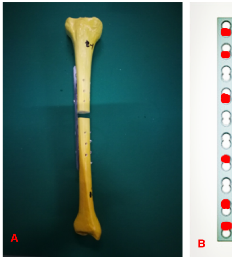
Fig. 1 Test construct design. a The titanium locking plates and CF-PEEK plates were evaluated in a standard plating configuration in tibial diaphysis surrogates with a 10-mm fracture gap as comminuted fracture. b The plate was applied with three locking screws, which were placed in the first, second, and fourth holes in each side (red spots)
