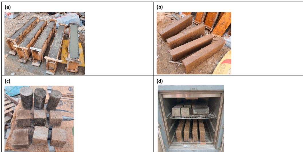
Fig. 8. Casting and curing process for all specimens. (a) Beams immediately after casting. (b) GPC Beam after 24 h from casting. (c) Cubes specimens after 24 h from casting. (d) Curing of specimens in the dry oven.
