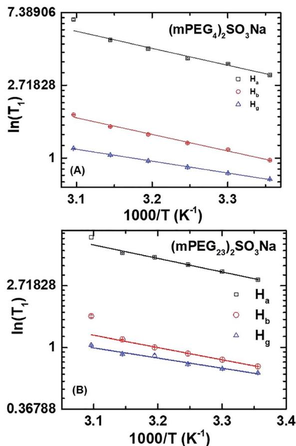
Fig. 4 Variable-temperature  $T_1$  data for (A) (mPEG<sub>4</sub>)<sub>2</sub>SO<sub>3</sub>Na and (B) (mPEG<sub>23</sub>)<sub>2</sub>SO<sub>3</sub>Na; the solid line represents the best Arrhenius fit of the experimental data described by the eqn (1).
