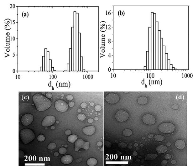
**Fig. 5** Upper panel: Size distribution histograms of aggregates in 2.0 mM solutions (pH 7) of (a) (mPEG<sub>4</sub>)<sub>2</sub>SO<sub>3</sub>Na, and (b) (mPEG<sub>23</sub>)<sub>2</sub>SO<sub>3</sub>Na at 25 °C; lower panel: unstained HRTEM images of 2 mM (c) (mPEG<sub>4</sub>)<sub>2</sub>SO<sub>3</sub>Na and (d) (mPEG<sub>23</sub>)<sub>2</sub>SO<sub>3</sub>Na solutions in phosphate buffer (pH 7.0).
