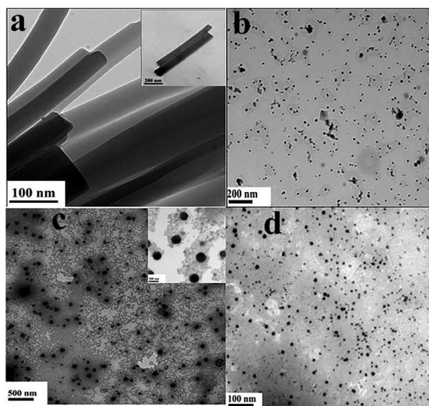
Fig. 8 HRTEM images of 5 mM  $(\text{mPEG}_4)_2\text{SO}_3\text{Na}$  containing (a) 200 mM NaCl, (b) 100 mM L-lysine hydrochloride; and 5 mM  $(\text{mPEG}_{23})_2\text{SO}_3\text{Na}$  containing (c) 200 mM NaCl, (d) 5 mM 100 mM L-lysine hydrochloride; inset (a): one section analysis; inset (c): one section analysis.
