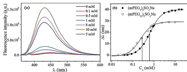
Fig. 3 (a) Representative fluorescence spectra of NPN in pH 7 buffer containing different concentrations of  $(\text{mPEG}_4)_2\text{SO}_3\text{Na}$ ; (b) plots of spectral shift ( $\Delta\lambda = \lambda_{\text{max,water}} - \lambda_{\text{max,sample}}$ ) of NPN as a function of  $C_s$  for  $(\text{mPEG}_4)_2\text{SO}_3\text{Na}$  (■) and  $(\text{mPEG}_{23})_2\text{SO}_3\text{Na}$  (□) in pH 7 buffer at 25 °C.
