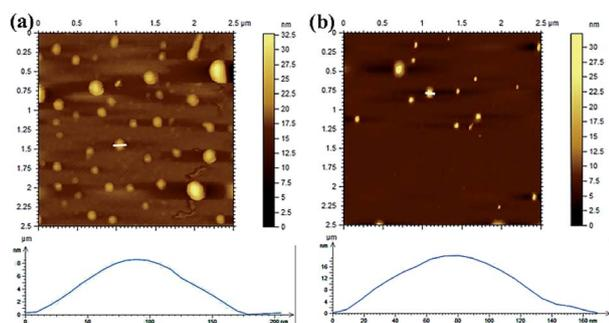
Fig. 6 AFM images (upper panel) with scale-bar and height distribution (lower panel) of the aggregates in 2 mM solutions of (a)  $(\text{mPEG}_4)_2\text{SO}_3\text{Na}$  and (b)  $(\text{mPEG}_{23})_2\text{SO}_3\text{Na}$  in pH 7.0.
