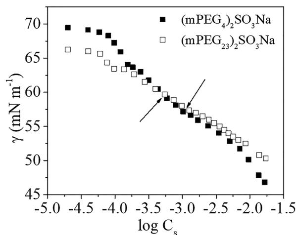
Fig. 2 Plots of variation of surface tension ( $\gamma$ ) phosphate buffer (20 mM, pH 7) as a function of  $\log C_s$  at 25 °C: (■) (mPEG<sub>4</sub>)<sub>2</sub>SO<sub>3</sub>Na, (□) (mPEG<sub>23</sub>)<sub>2</sub>SO<sub>3</sub>Na.
