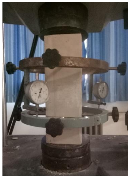
Figure 2. Elastic modulus test of prism.
