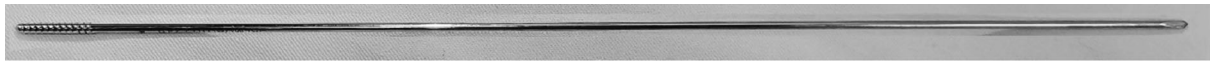
Fig. 1 Physical diagram of thread elastic intramedullary nail. The diameters of the TEIN can be divided into 1.5 mm and 2.0 mm, with a length of 260 mm. TEIN is made of stainless steel (317 L). The nail head end is a positive cone, followed by a thread with 15–20 mm length and height higher than the 1.0 mm of the nail body, and the nail body has a certain elasticity.
