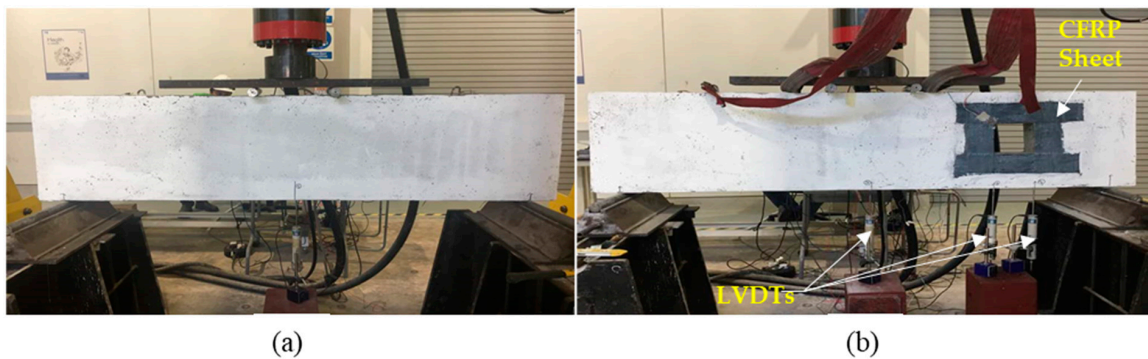
Figure 4. Equipment and testing setup: (a) control beam; and (b) deep beam with opening.
