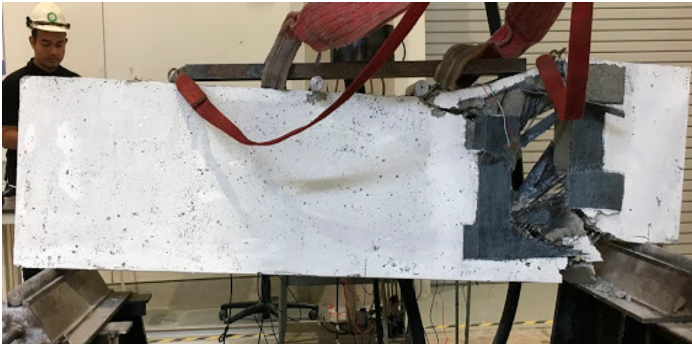
Figure 9. Failure mode and cracking pattern of deep beam B2a.
