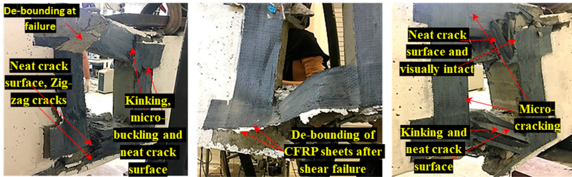
Figure 15. Typical post-mortem photos after the static four-point bending tests of the deep beams with opening.
