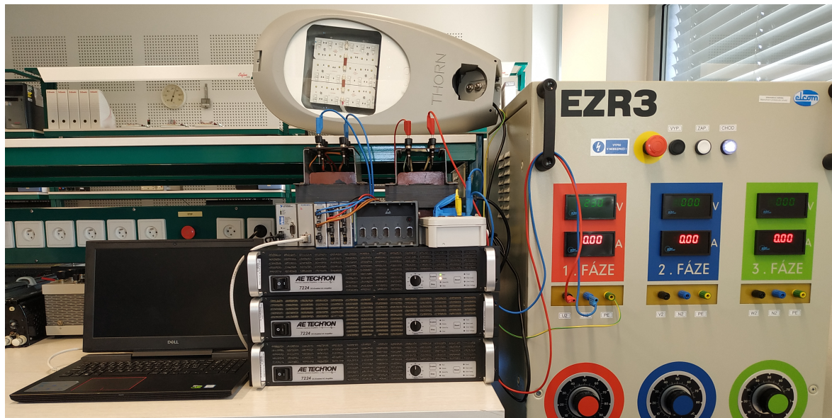
Figure 21. Realized laboratory experiment with AE-Techtron 7224 amplifiers used as inverters.
