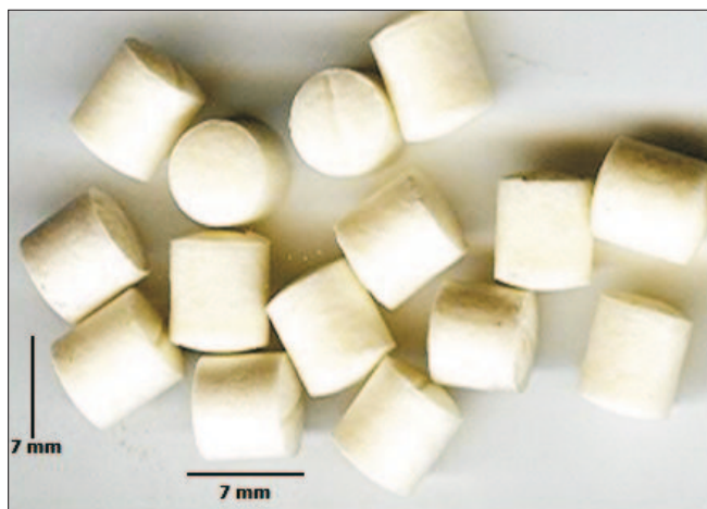
Fig. 1: Cefoperazone sodium impregnated calcium sulphate-polycaprolactone composite pellets
