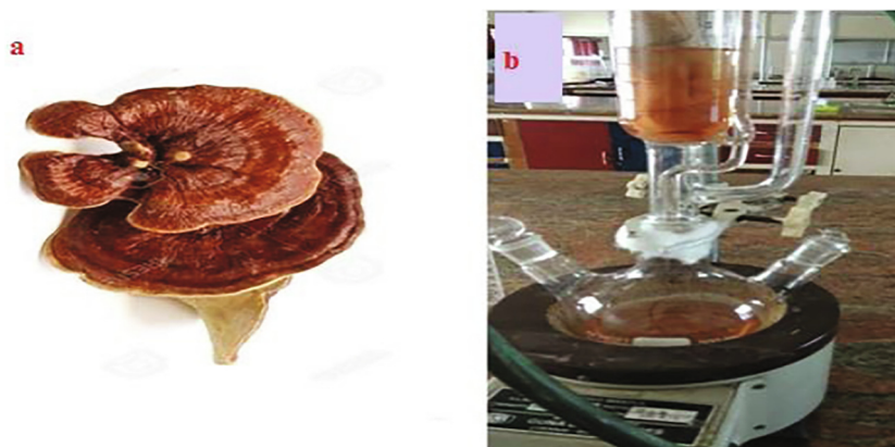
Fig. 1. (a) G. lucidum (Basidiomycota Fungi); (b) Ethanolic extract of G. lucidum using Soxhlet apparatus.
