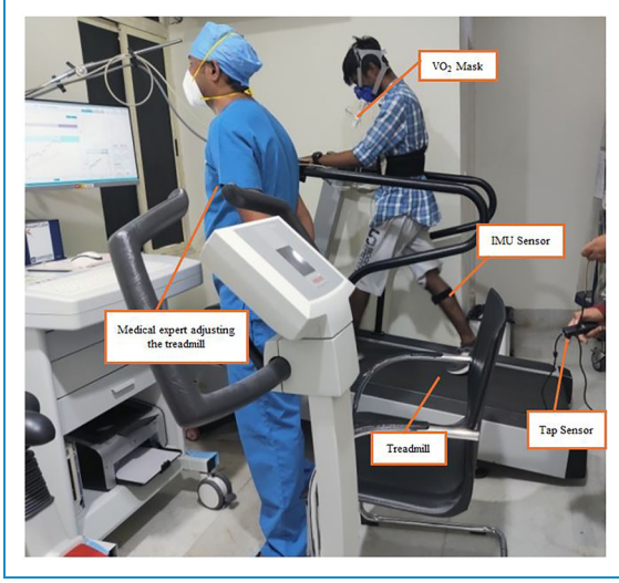
Figure 5. Subject wearing VO 2 mask (middle), a medical expert is adjusting the treadmill using Bruce protocol (left side of image) and doctor who is operating manual push button (right side of image).
