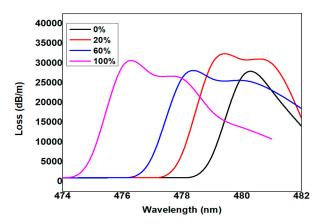
**Figure 2.** Loss spectra versus wavelength with respect to the variation of the alcohol concentration keeping Ag as 30 nm.
