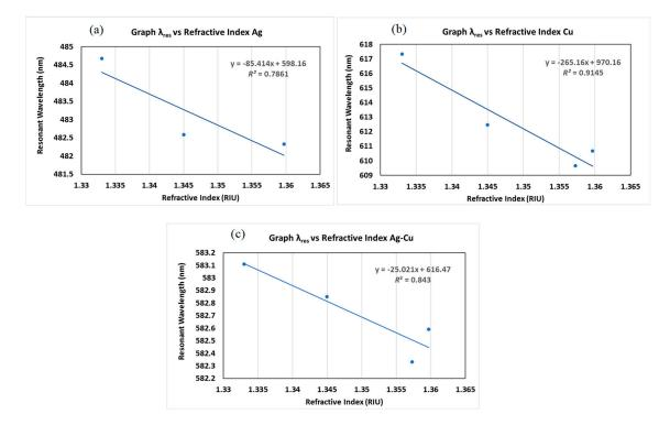
**Figure 9.** Graph of resonance wavelength against the refractive index for (**a**) Ag, (**b**) Cu, and (**c**) Ag–Cu bimetallic combination.
