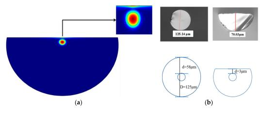
**Figure 1.** The cross-sectional view of the bimetallic D-shaped optical fiber at the coupling point of the metallic and core modes: (**a**) simulation model and (**b**) the dimensions of the D-shaped optical fiber from microscopy images.
