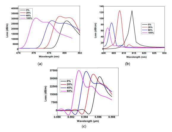
**Figure 3.** (a) Loss spectra versus wavelength with respect to the variation of the alcohol concentration keeping Ag as 30 nm. (b) Loss spectra versus wavelength with respect to the variation of the alcohol concentration keeping Cu as 10 nm. (c) Loss spectra versus wavelength with respect to the variation of the alcohol concentration keeping Ag and Cu thickness as 30 nm and 10 nm, respectively.
