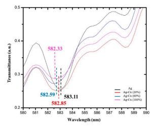
**Figure 8.** SPR sensor's transmittance spectra versus the wavelength for Ag–Cu shifts at different alcohol refractive indexes as (black line) Ag–Cu at 583.11 nm (red line) wavelength of Ag–Cu as 582.85 nm sensed at 20% of alcohol (blue line); 582.59 nm of Cu sensed at 40% of alcohol; and Cu sensed using 60% of the alcohol concentration at 582.33 nm (pink line).
