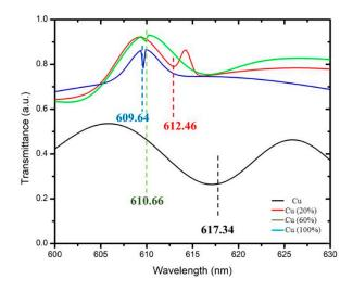
**Figure 7.** SPR sensor's transmittance spectra versus the wavelength for Cu shifts at different alcohol refractive indexes as (black line) Cu at a 617.34 nm (red line) wavelength of Cu as 612.46 nm sensed at 20% of alcohol (green line); 610.66 nm of Cu sensed at 40% of alcohol; and (blue line) of Cu sensed using 60% of the alcohol concentration at 609.64 nm.
