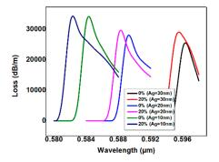
**Figure 4.** Variation of loss spectral shift for the bimetallic thickness of Ag = 30 nm, 20 nm, 10 nm under the constant thickness of Cu = 10 nm.
