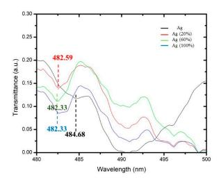
**Figure 6.** The surface plasmon resonance (SPR) sensor's transmittance spectra versus the wavelength of Ag wavelength shifts at different alcohol refractive indexes, where (black line) Ag at a 484.68 nm (red line) wavelength of Ag 482.59 nm sensed at 20% of alcohol (green line); 482.33 nm of Ag sensed at 60% of alcohol; and (blue line) Ag sensed at 100% of alcohol concentration placed at the same wavelength as 60% of the alcohol at 482.33 nm.
