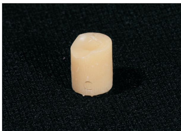
Figure 7. Clinical image of a fractured specimen showing a cohesive fracture.
