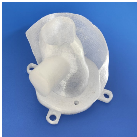
Fig. 2 Multi-sectional image of the real 3D printed LVm defective phantom
