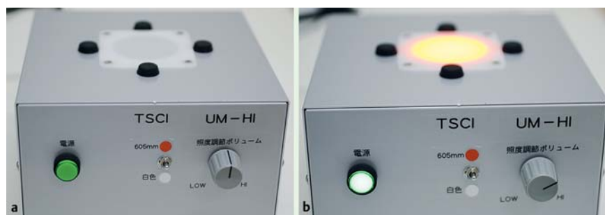
Fig. 1 We developed a device equipped with a 605-nm wavelength light source, referred to as the target sample check illuminator (TSCI).
