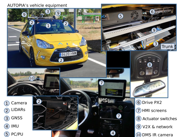
Figure 15. Modules of the autonomous vehicle of AUTOPIA Program.
