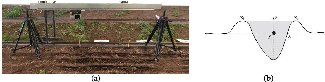
Figure 3. The LiDAR-based soil surface measurement unit in the semi-field facility (a); Sketch of the furrow geometry that includes the reference frame of the cross-sectional profile (b), solid line indicates the soil surface and dashed lines indicate the vertical and horizontal axis of the origin.
