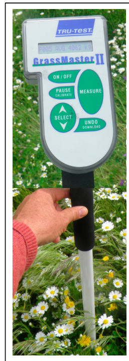
Figure 8. Grassmaster II electronic capacitance probe used to estimate pasture biomass.
