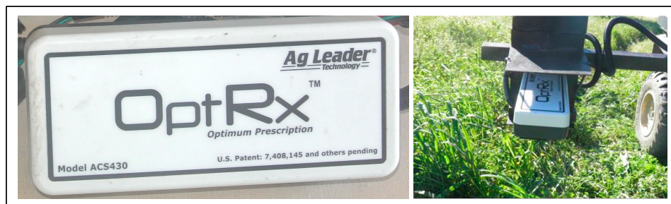
Figure 9. Active optical sensor “OptRx™” used to measure NDVI.
