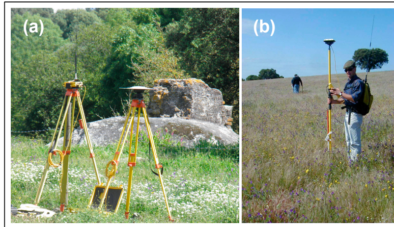
Figure 3. Trimble RTK/PP-4700 GPS: (a) station and radio; (b) rover.
