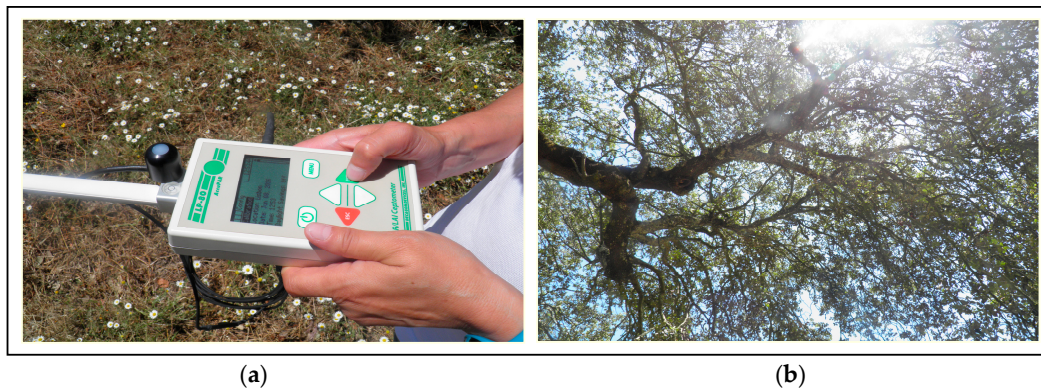
Figure 6. Ceptometer AccuPAR LP-80 (a) used to measure the photosynthetically active radiation (PAR) (b).
