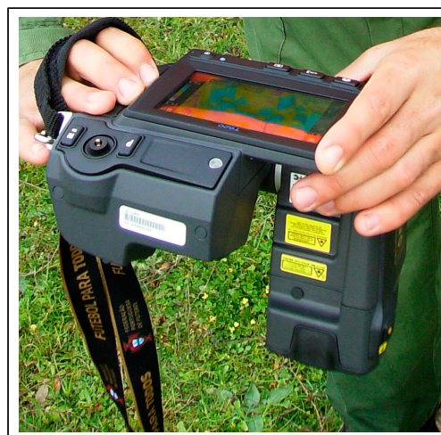
Figure 7. ThermaCAM™ infrared camera used to measure the temperature at the pasture surface.
