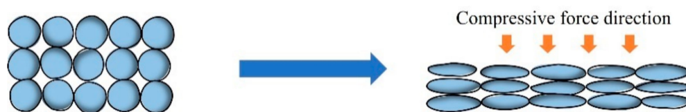
Figure 6. Viscoelastic behavior and compact structure of PSS/PDADMAC PEC hydrogels by compressive force.
