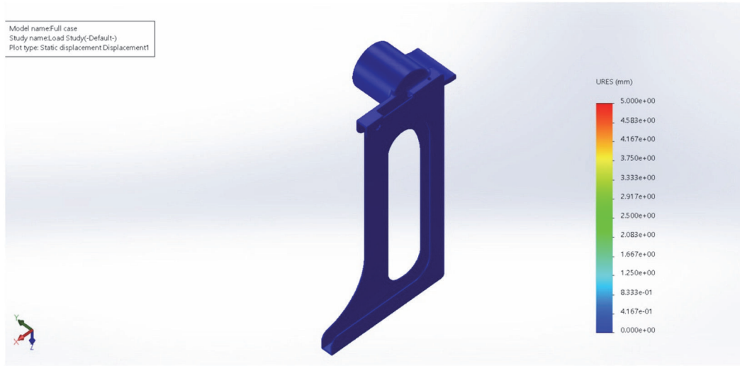
FIGURE 8: Static displacement plot (we can see that for a load of 200 gms the maximum displacement is no more than 0.02 mm).
