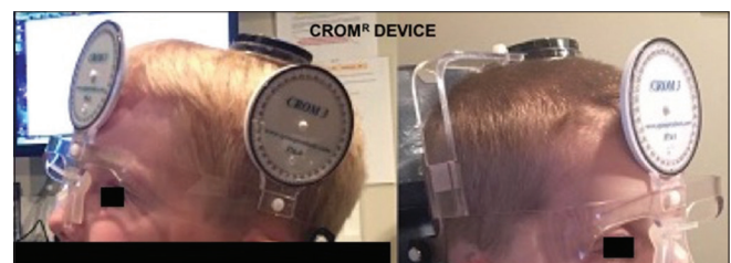
Figure 1: Cervical Range of Motion ® Device. Photograph illustrating measurements of head posture used to collect anomalous head position data. The device is placed on the head prior to visual acuity testing. The instrument ensures accurate determination of the head position (eccentric null zone position) in pitch, yaw, and roll during routine binocular best-corrected distance acuity testing
