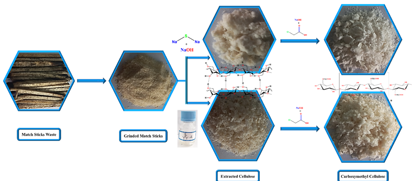
Figure 1. Schematic representation of the overall extraction of cellulose from matchstick waste and conversion into CMC.
