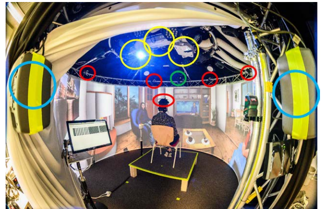
Fig. 2. Virtual reality lab at Oldenburg University (photo: Hörtech gGmbH). Projectors (yellow) project a 300-degree field-of-view image on a cylindrical screen. Sound is rendered over a spherical multi-loudspeaker array with 29 full-range loudspeakers (blue) and 4 subwoofers. Sensors include EOG sensors for eye gaze, EEG sensors, and head tracking (red). Furthermore, the subject can be video recorded during an experiment (green). EEG indicates electroencephalography; EOG, electrooculography.
