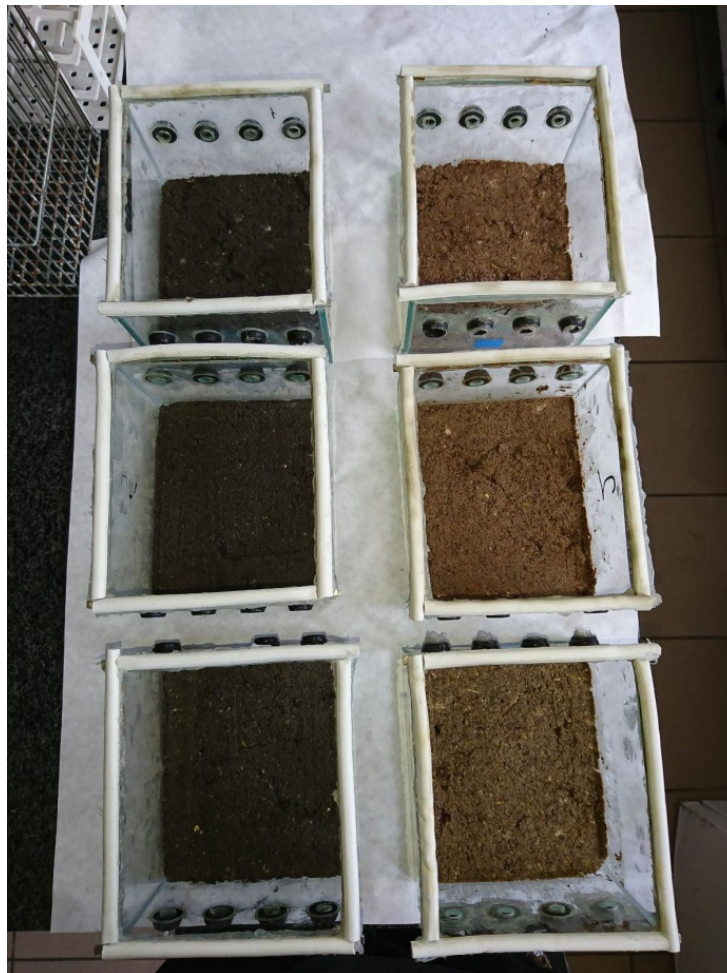
Figure A4. Glass containers with poultry litter used for \text{NH}_3 emissions evaluation.
