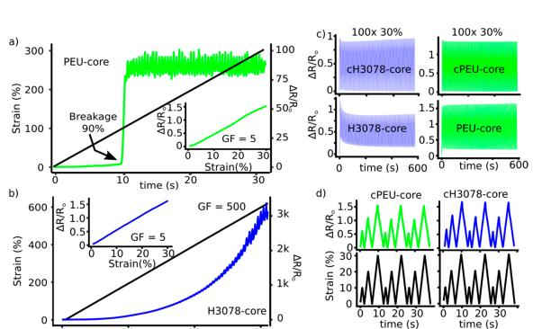
**Figure 4.** (a) PEU core sensor piezoresistive limit and sensor linearity up to 30% strain (inset); (b) H3078 core sensor piezoresitive limit and sensor linearity up to 30% strain (inset); (c) 100 repetitions of 0–30% strain for pristine H3078 core, PEU core, cH3078 core, and cPEU core sensors; (d) 10%, 20%, and 30% trapezoid strain for three cycles with cPEU core and cH0378 core sensors.
