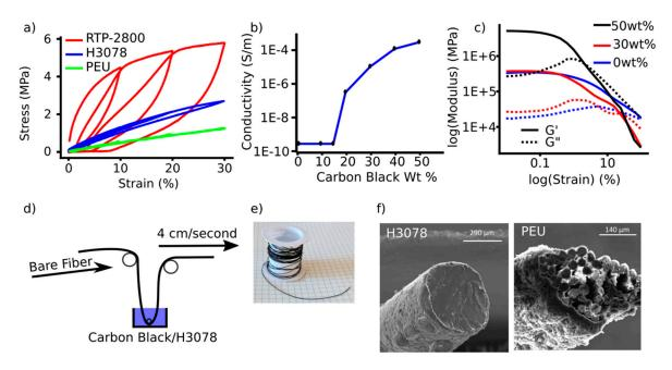
**Figure 3.** (a) Stress–strain curves for RTP-2800, H3078, and PEU; (b) Percolation threshold for carbon black in H3078; (c) Rheological amplitude sweep for carbon black loading in H3078; (d) Schematic for the dip-coating process of H3078 and PEU cores; (e) Resulting conductive fiber (H3078 core shown); (f) SEM image of core–sheath H3078 and PEU core sensors.
