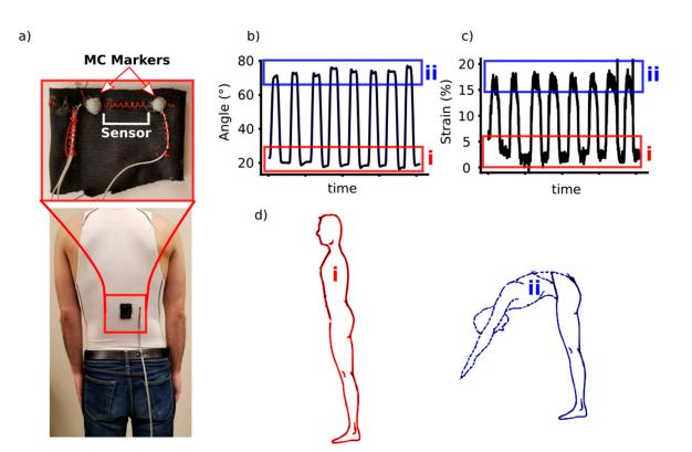
**Figure 1.** (**a**) A sample patch with motion capture markers fixed to an undershirt and worn to obtain the following values; (**b**) Angles obtained from a standing static position (i) to forward bending (ii); (**c**) Strain that is observed when going from a static standing position (i) to forward bending (ii); (**d**) static standing position (i) and forward bending (ii) completed for (**b**) and (**c**).
