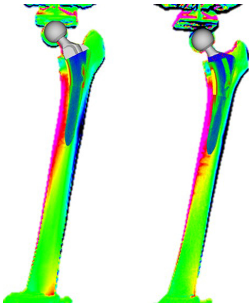
Figure 11 Contact sites and stress distribution (Left: synthetic bone 1, Right: synthetic bone 2)
