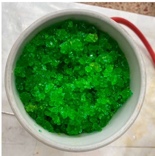
Figure 1. Ferrous chloride crystals obtained from water pickling liquors by the described method.
