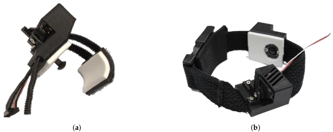
Figure 4. (a) Mechanotactile factors on forearm mounting system. (b) Mechanotactile factors on fingertip mounting system.
