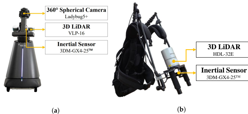
Figure 8. (a) Robot system and (b) backpack system employed for data acquisition.
