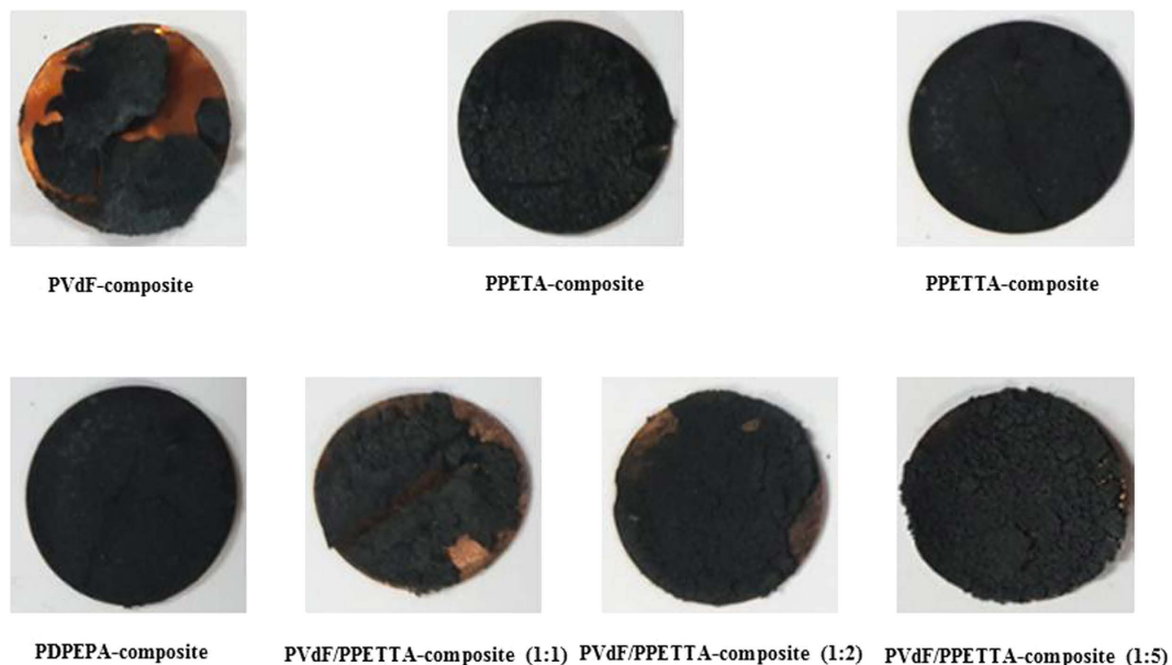
Figure 5. Images of the PVdF-composite, PPETA-composite, PPETTA-composite, PDPEPA-composite and PVdF/PPETTA-composites after 10 cycles.
