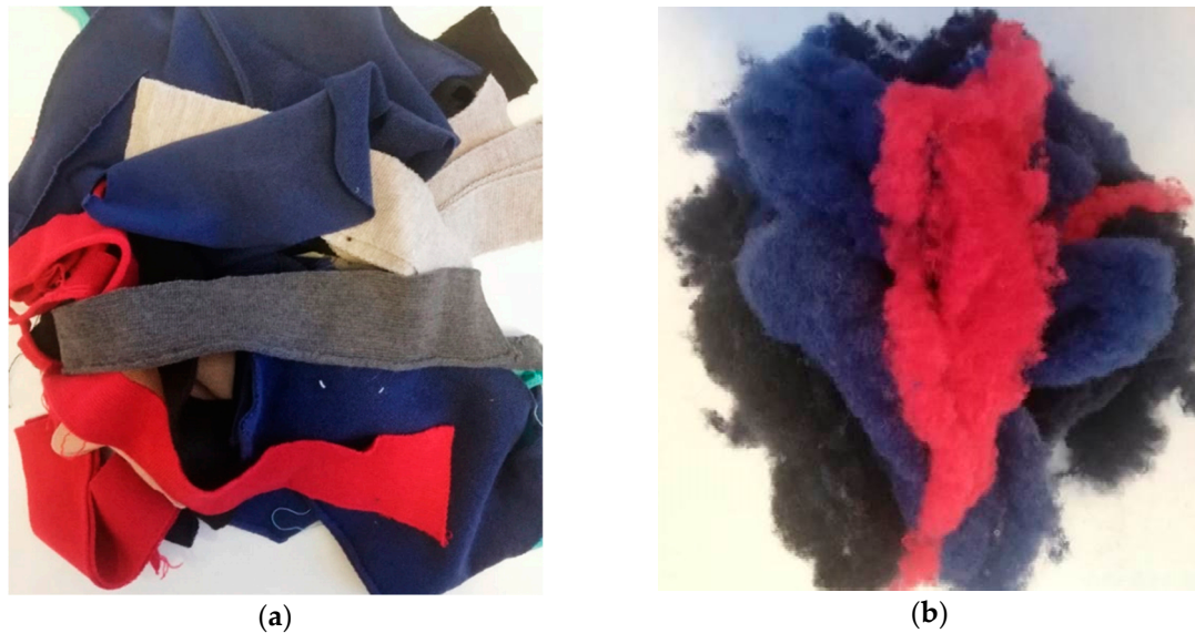
Figure 1. Textile waste in the form of cut fabrics (a) and fleece matrix used as raw material (b).
