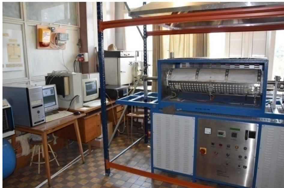
**Figure 1.** Laboratory stand for testing reductions in a rotary furnace after the upgrade [26].
