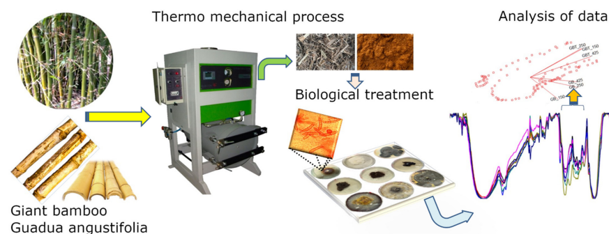
Figure 1. Eco-friendly proposal to modify the chemical structure of lignocellulosic compounds and break down the lignin linkages in natural fibers.
