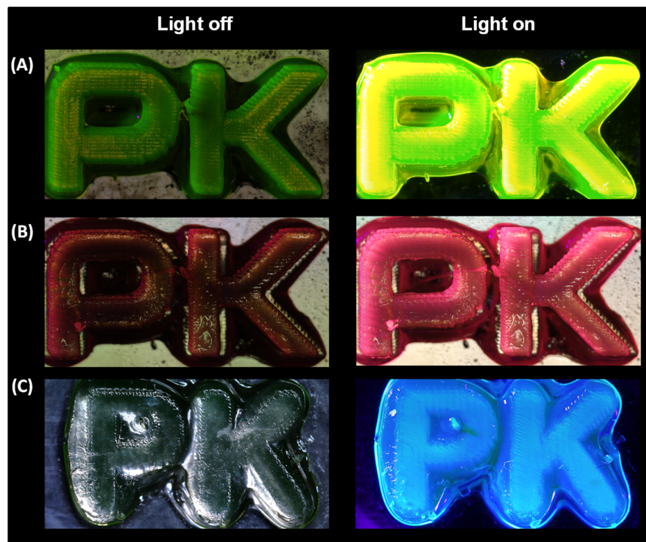
Figure 4. Print comparison obtained by NEJE laser engraver printer. Comparison was made with light off and light on for: (A) BODIPY; (B) Eu1; and (C) Coumarin 1.
