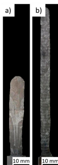
Figure 6. Macrostructure of samples produced: (a) with secondary heat source and (b) without (adapted from [34]).
