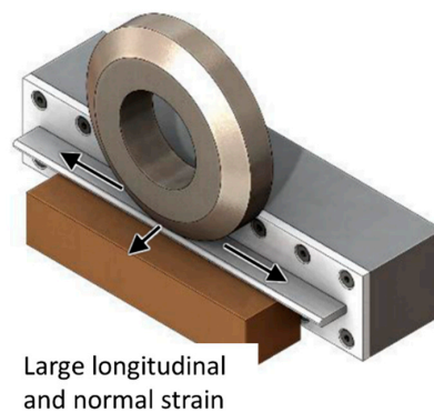
Figure 3. Schematic representation of side rolling of WAAM part to enhance surface finish (adapted from [19]).
