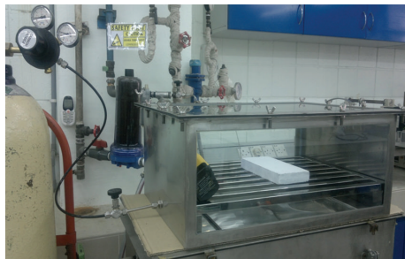
FIGURE 3: LiNbO 3 coated concrete slab in reaction chamber.
