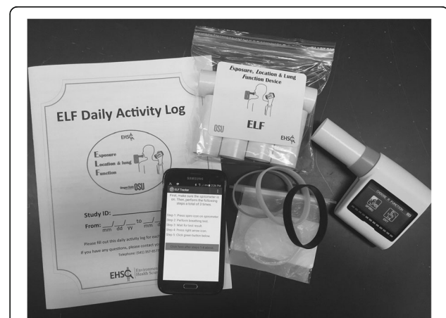
Fig. 1 Photograph of the ELF components. Clockwise from left: Activity log for self-reported environmental exposures, disposable paper mouthpieces for use with the hand-held spirometer, 7 silicone wristbands in air-tight packaging, and an Android phone hosting the ELF Tracker
