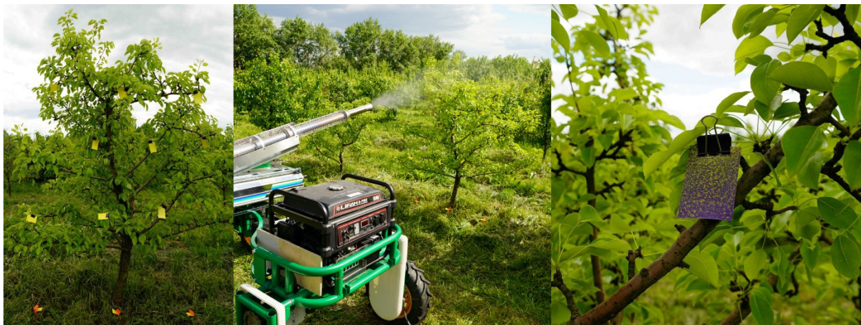
Figure 4. Pieces of water-sensitive paper fixed on a tree after contact with drops of aqueous PPP solution.
