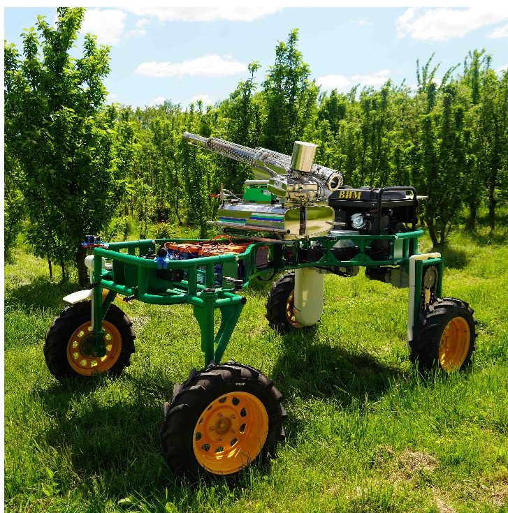
Figure 3. Automated platform with an aerosol mist generator installed.
