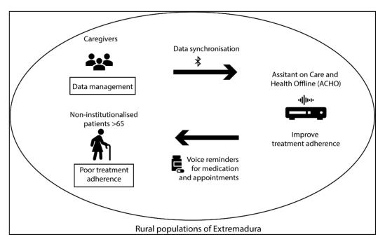
Figure 8. ACHO operational diagram: Bluetooth connection and current functionalities.
