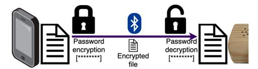
Figure 7. Synchronisation process following symmetric encryption.
